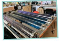
A few year 10ns and me got invited to a solar factory to see how solar panels are made and how they can change the future. They showed us a new style of solar panels. The solar panels where in a glass tube also they can warm up water as well.
